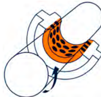
Fig. 1 Self-lubricating bearing in contact with the shaft
